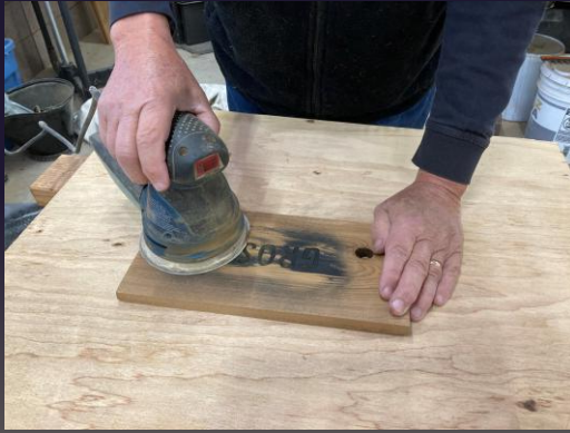
Sanding to Remove Paint
